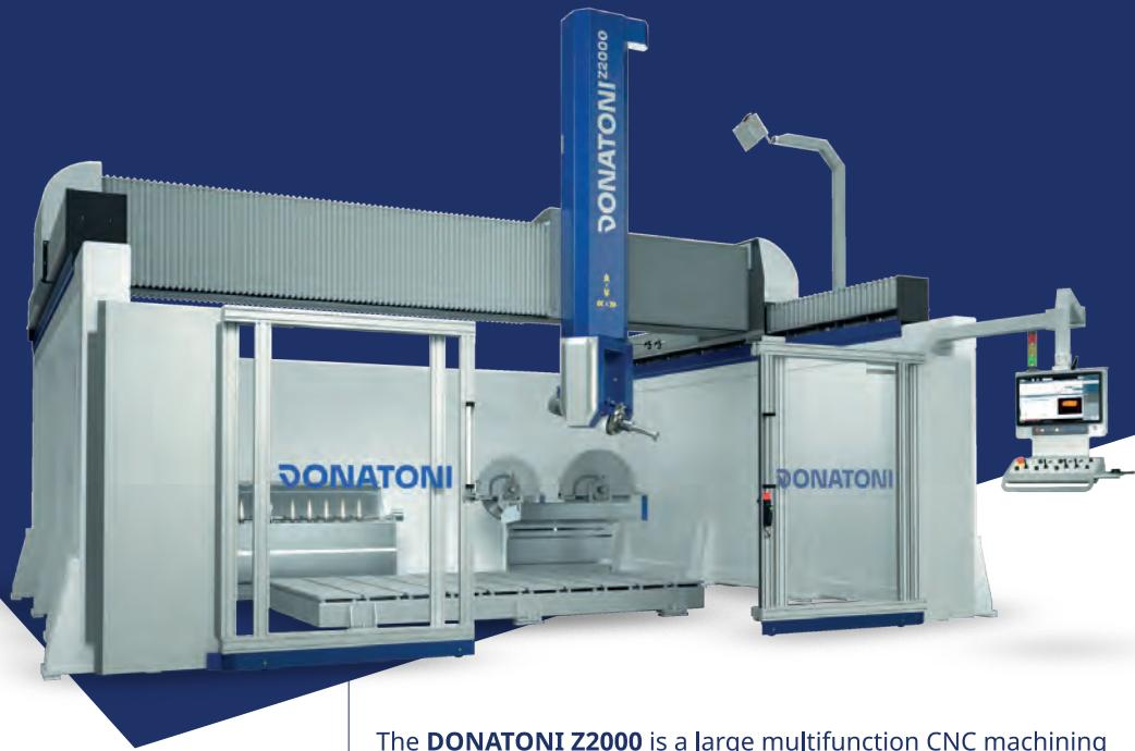
The **DONATONI Z2000** is a large multifunction CNC machining centre with **5/6 interpolated axes with a Z axis stroke of 2000 mm**. It is suitable for shaping operations (simple and complex, rectilinear, concave, convex, arched), for milling two- and three-dimensional sections, as well as for making columns, sculptures, and all types of cuts.
